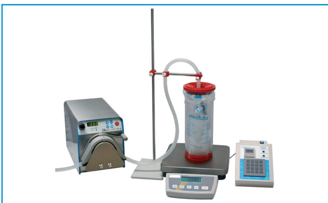
Figure 13: Smart Dispenser - high precision boar semen dilution
